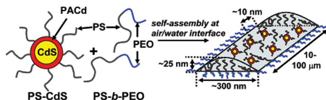
Scheme 2. Cooperative Self-Assembly of PS-CdS and PS- b -PEO at the Air–Water Interface
